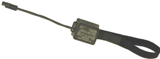
The **Multi Chemistry Charger** connects directly to a Power Input. It will charge both Li-Ion and NiMH batteries, although charge times will be greater than with the **Charge Controller**. The **Multi Chemistry Charger** only charges batteries and does not provide pass-thru power.
