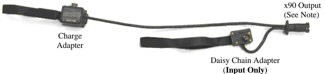
The *Pass-Thru Assembly* can be used to power a device while charging a battery. Note a battery must be connected to the charge adapter of the *Pass-Thru Assembly* in order to get pass-thru power. Also note the *Daisy Chain Adapter* is INPUT ONLY, and will not charge a battery. The *Charge Adapter* is connected to output pins 1 & 4, while the *Daisy Chain Adapter* is connected to output pins 2 & 5.
